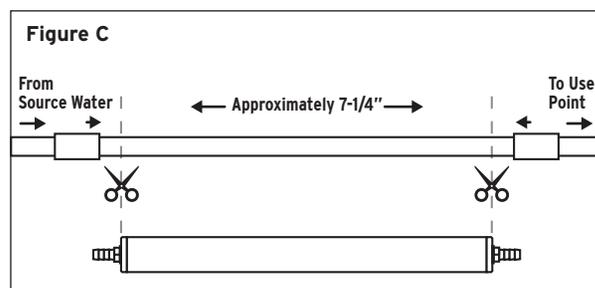
3. Cut the tubing at the marks using a tubing cutter, sharp knife, or scissors.
