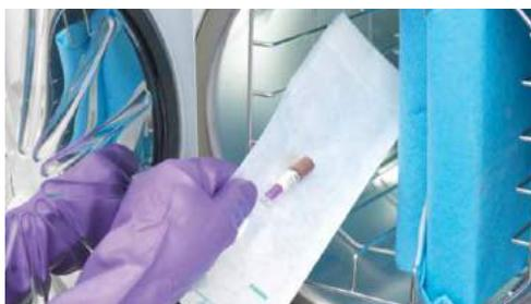
Assuming this strip is brown, after 10 minutes' cooling time has elapsed, both the test and the control vials are crushed and placed in the incubator for 24 hours. The operator can then view the color of the liquid in the test and the control vials – if the culture medium is still purple while the control test's culture medium is yellow, the test is negative, indicating sterilization occurred. If the color is yellow, the test is a fail (growth of spores has occurred during incubation).
