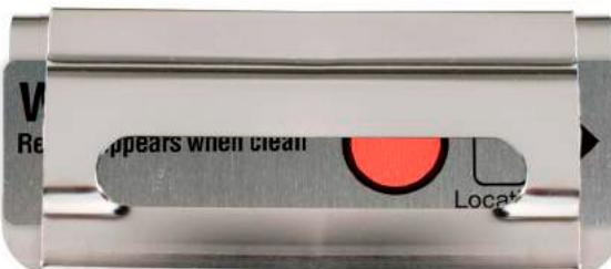
Spray is blocked in the upper area, requiring in-direct impingement of cleaning solution to reach the test soil.
