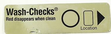
Figure 5. Complete removal of red test soil on Washer-Disinfector Cleaning Monitor after cleaning instruments at Hydrim P3-Heavy Duty Cleaning Cycle.
