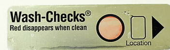
Figure 6. Residual red test soil on Washer-Disinfector Cleaning Monitor after blood-coated instruments were exposed to P1 Rinse-Hold Hydrim cycle.
