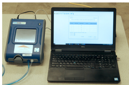
PortaCount® Pro+ Respirator Fit Tester (TSI) and screen results
