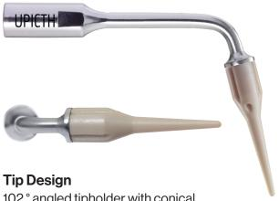
102° angled tipholder with conical implant cleaning tip (working length 10 mm, Ø apical 0,8 mm, Ø coronal 2 mm)
