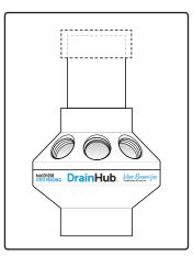
1-1/2" Pipe or Tube Stack (Open or Capped)
