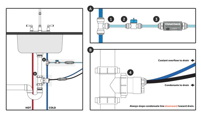
Connect the system to cold water supply ahead of foot switch (if present) for uninterrupted water supply.
