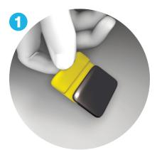
Place wireless sensor or plate in barrier sleeve (not included). Insert sensor into Slip-Ease<sup>™</sup> Comfort Cushion.
