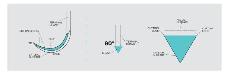
When sharpening either the straight or curved sickle scaler you will restore the cutting edges by grinding against the lateral surfaces of the blade and finishing the facial surface. Excessive sharpening of the facial surface is not recommended because it will weaken the blade.
