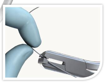
Step Pliers help to create a right-hand or left-hand step-up or step-down in wire at 1/2 mm, 3/4 mm or 1 mm intervals.
