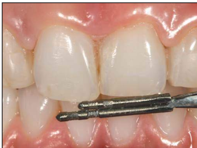
Figure 1. Prototype proportion gauge; a Siamese twin instrument tip with preset markings notched into the surface with measurements indicating a predetermined 78% width to length proportion.
